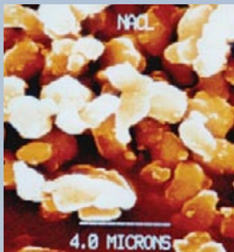
Scanning electron microscope image of experimental hygroscopic powder milled to the optimal size of 2 to 5 microns, used in a seeding experiment conducted in parallel in Israel and Texas (from D. Rosenfeld).
