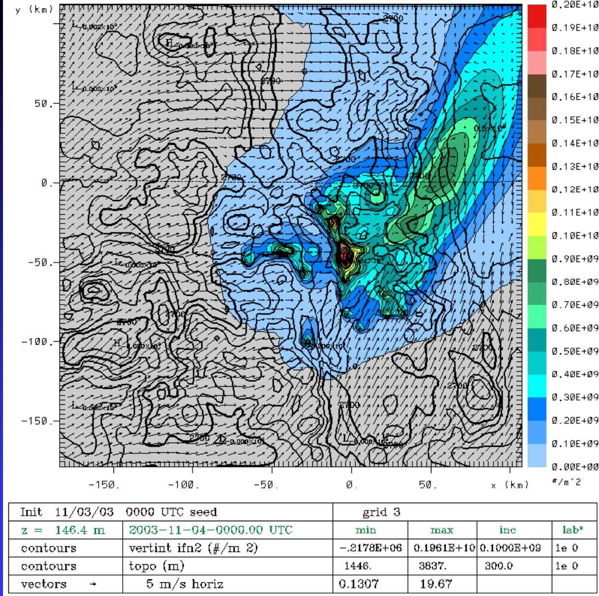
Vertically integrated available seeded IFN concentration. Shows both the generator sources and the advected downwind plume.
