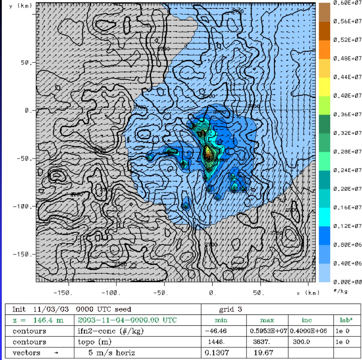
Available seeded IFN concentration in lowest model level. The approximately 15 small maxima indicate the source grid points where active seeding generators are located.
