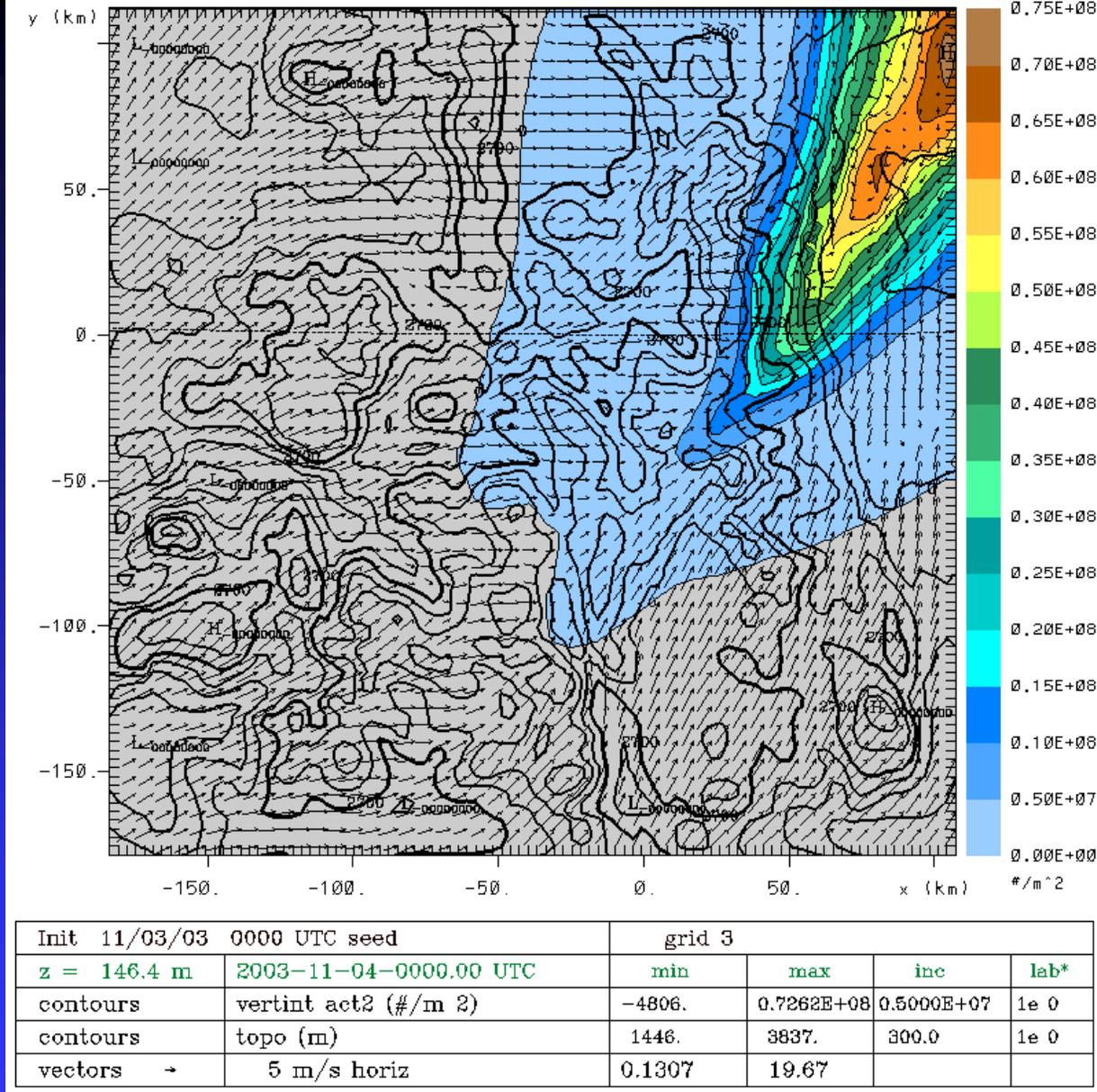
Vertically integrated activated seeded IFN concentration (contributes to pristine ice concentration along with activated background IFN). The activated seeded plume is primarily downwind of the Target Area to the lee of the Front Range.
